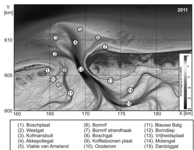
**Figure 1: Morphological state of the Ameland inlet in 2011 (Elias et al. 2013)**
