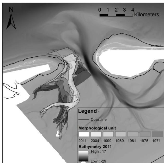
**Figure 4: Dynamics of the Boschgat at -3 m+NAP**
