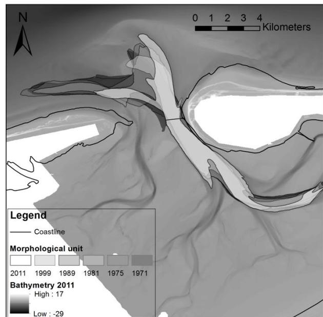
**Figure 2: Dynamics of the Akkepollegat and Borndiep at -8 m +NAP**
