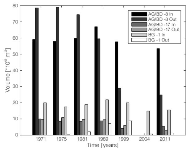
**Figure 3: Volume of the channel (the numbers show the height of the contour line [m +NAP], 'In' means inner delta, 'Out' means outer delta, 'AG/BD' means Akkepollegat combined with Borndiep and 'BG' means Boschgat)**
