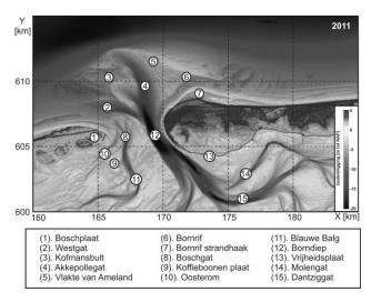
Figure 1: Morphological state of the Ameland inlet in 2011 (Elias et al. 2013)
