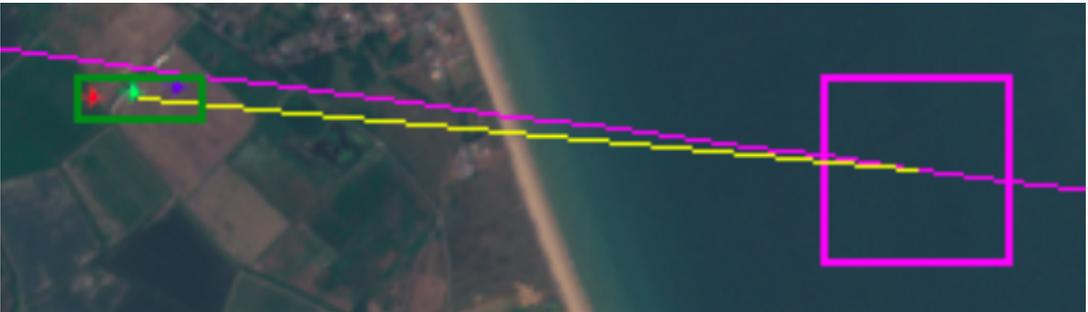
**Figure 1.** Sentinel-2 true color image of the southeast part of England. The magenta box indicates the interpolated ADS-B signals (magenta line) to the image sensing time. The aircraft annotation is indicated by the green box. The yellow line indicates the association of the ADS-B signals to the aircraft. See the text for an explanation of aircraft color displacement.
