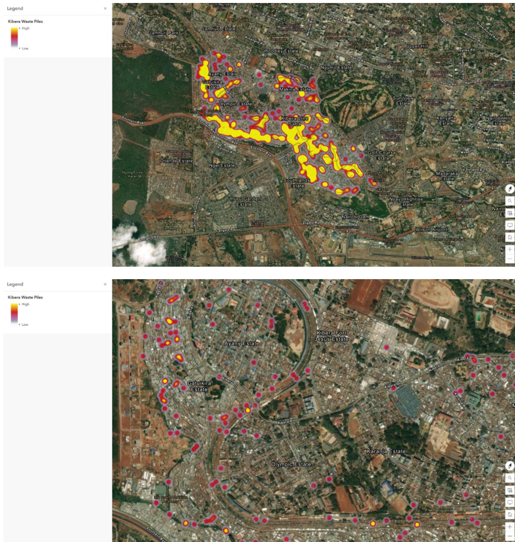
Figure 2 and 3. Visualisation six, heat map overlay of the Kibera DUA. (Top) Zoomed out and (Bottom) zoomed in towards the North West of the DUA. Yellow colour represents the higher volume of waste and red the smaller volume. When zoomed out, the entire DUA appears highly concentrated with waste. But zooming in shows far more spread of waste.
