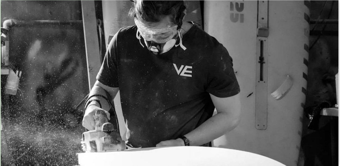
Figure 4: Shaping a surfboard's foam core. Photo by Sander van Eck, © 2022.
