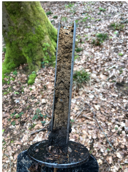
02 Soil sample taken in Lausanne using an auger. The black and brown colorations indicate the presence of carbon in the top 20 centimeters of the soil. Source: Photograph by the author
