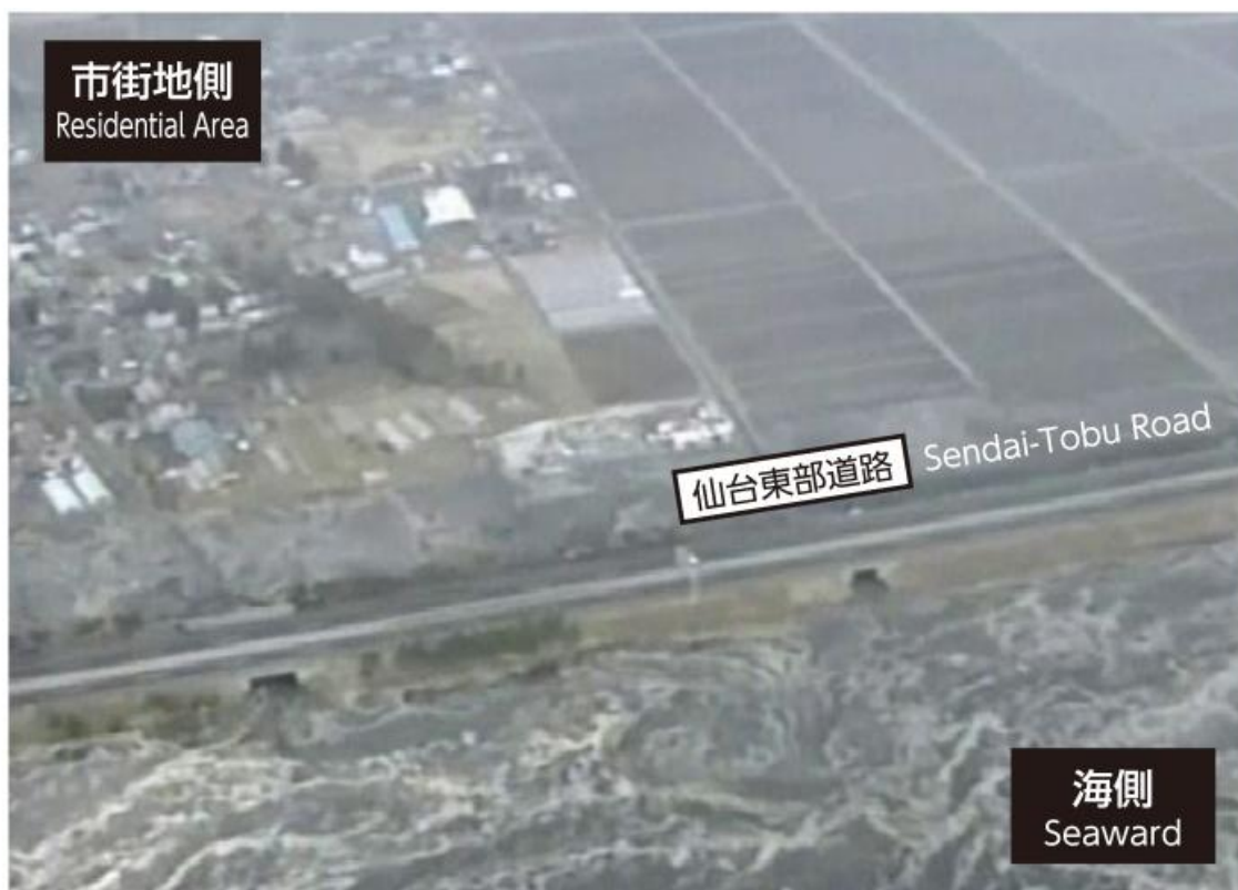
Figure 8. Photo from MLITT (2025) showing the 2011 tsunami primarily confined seaward of the Sendai Tobu road freeway embankment in Miyagi Prefecture.
