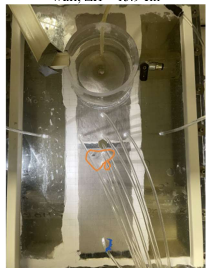
(l) Erosion failure occurred at the filter layer, \Delta H = 33.9\text{ cm} (constant)
