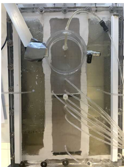
(a) Boiling sand phenomenon at the outlet, \Delta H = 1.1 cm
