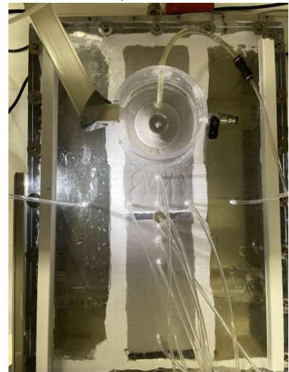
(i) Overall erosion in the downstream area of the cut-off wall, \Delta H = 15.9\text{ cm}
