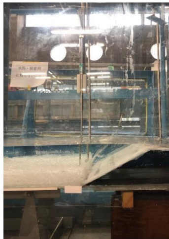
Figure 3: Appearance of polyethylene sheet in the wave flume
