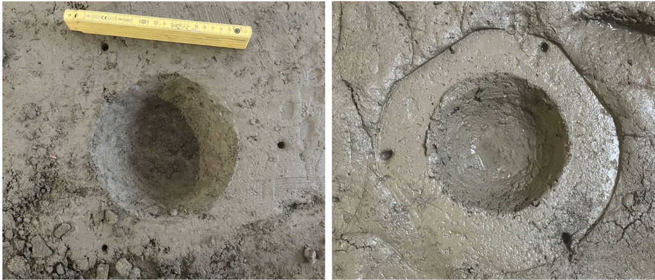
Figure 18. Imprint of field density measurement equipment on core soil from the same layer. To the left, the picture show very stiff core soil and very wet and soft to the right (Lagerlund and Riaz, 2026).
