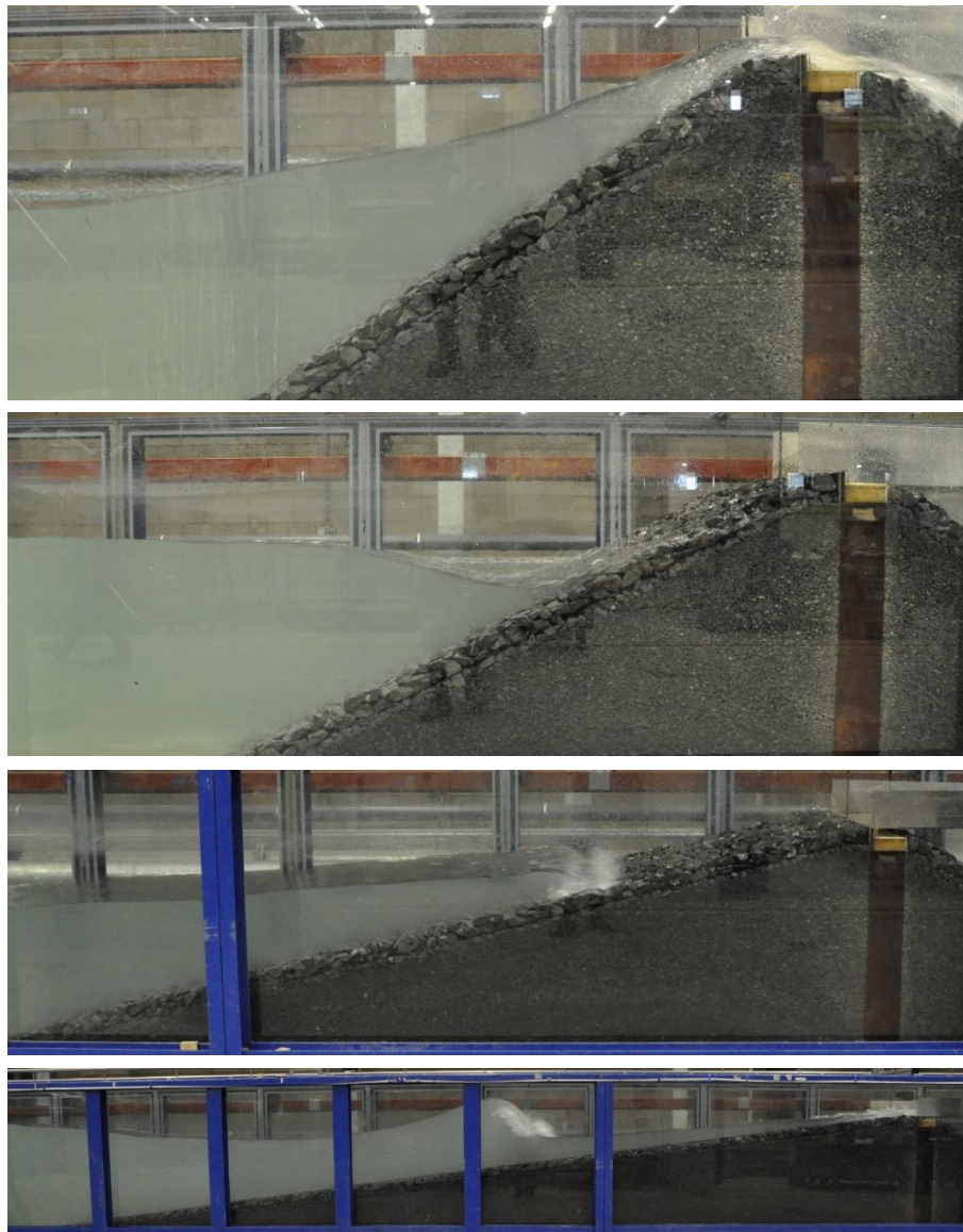
Figure 2: Pictures of wave action on a 1:1.5 slope, 1:2 slope, 1:4 slope and 1:8 slope, respectively.
