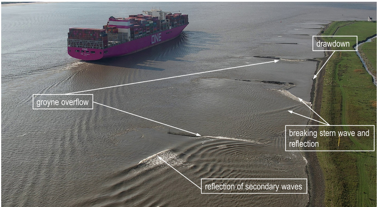
Figure 12: Complex wave interaction effects of long-period vessel wave with shallow groyne field and armoured embankment at Juelssand in the Lower Elbe Estuary, Germany. Source: Federal Waterways Engineering and Research Institute (BAW).
