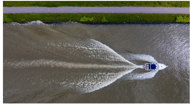
Figure 2: Interaction of short-period waves from recreational vessel with an embankment in an inland waterway. Source: Federal Waterways Engineering and Research Institute (BAW).
