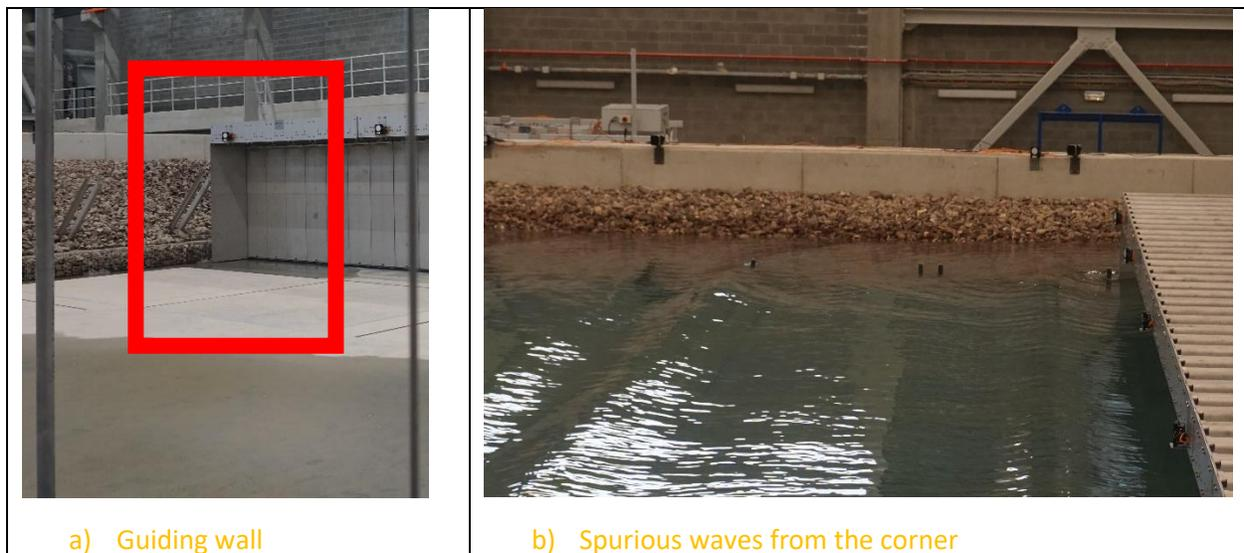
Figure B6. Guiding wall and the diffracted waves
