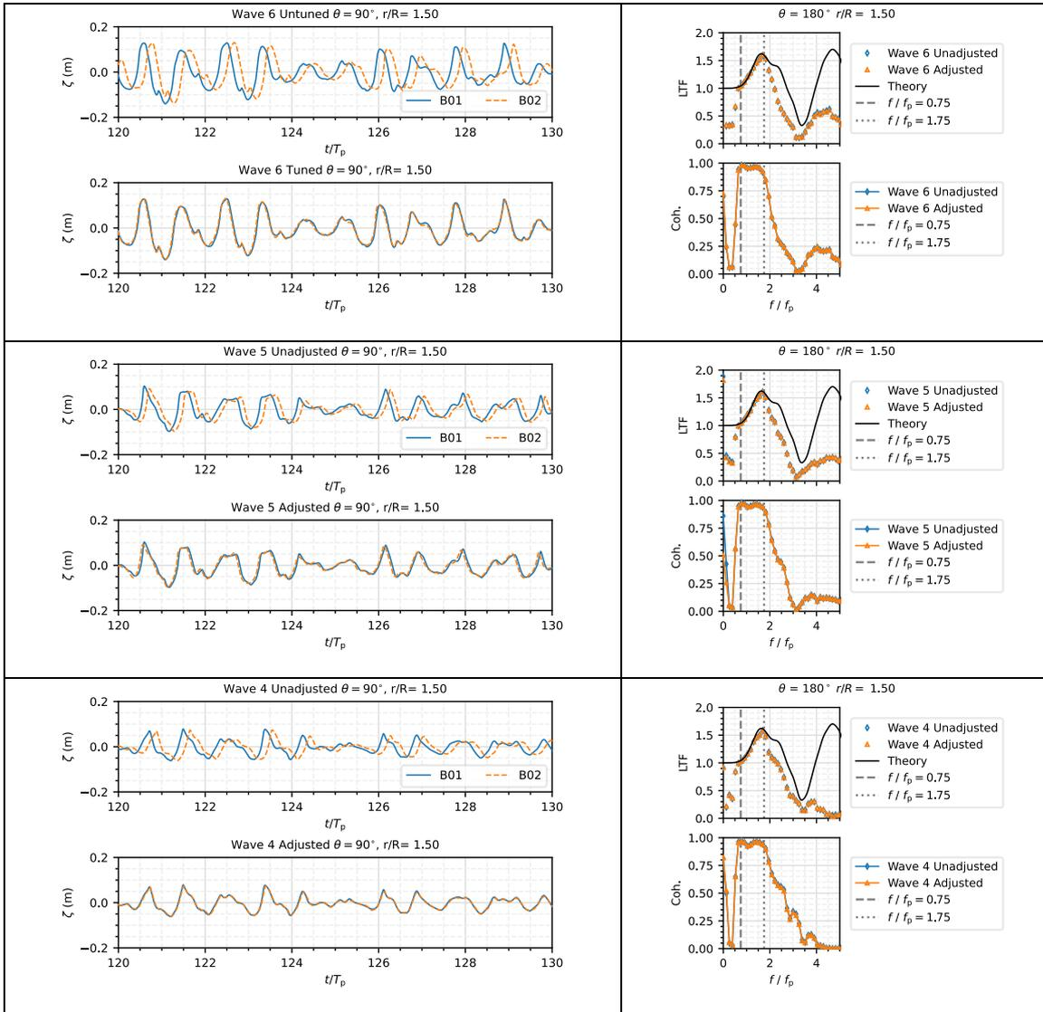
FIGURE D. Time shifting effect in the LTF estimation
