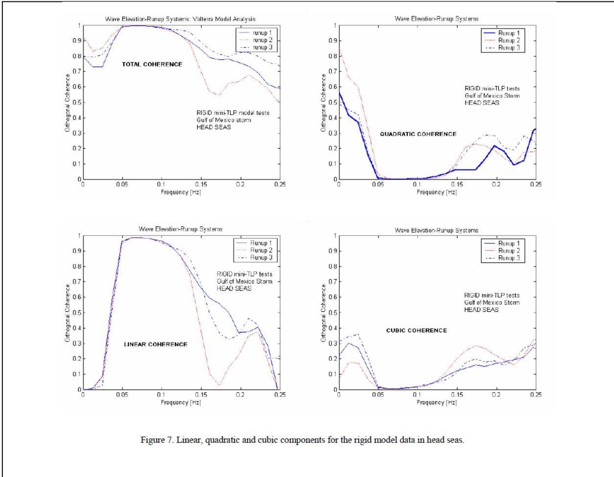
Figure 7. Linear, quadratic and cubic components for the rigid model data in head seas.
