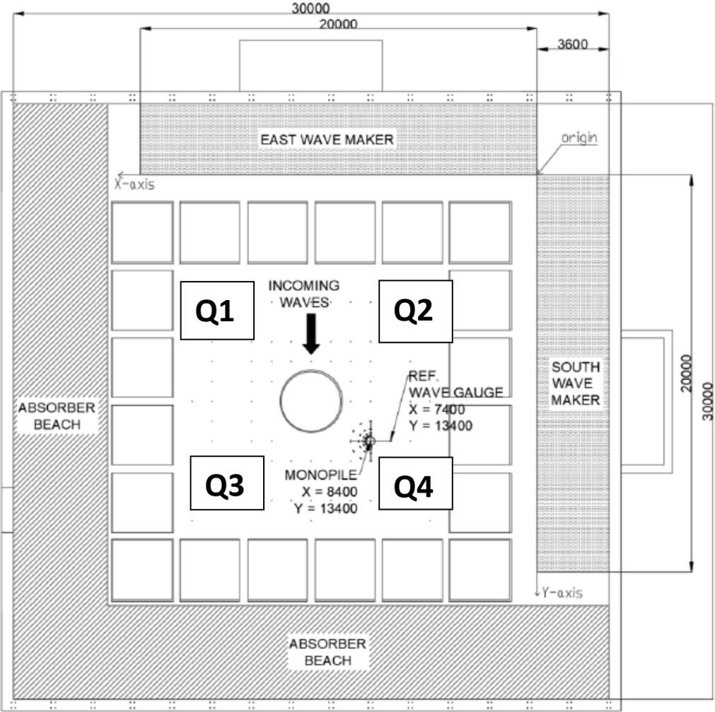
Figure B2. Quadrants division to select the most optimized spot of the COB basin.
