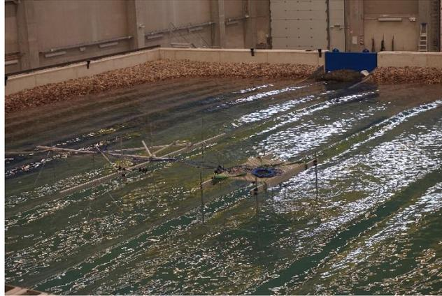
Figure B3. Bended wave crest due to the basin absorber beach.
