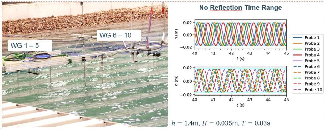
Figure B5. Wave arrangements and the measurements of the Arrangement B
