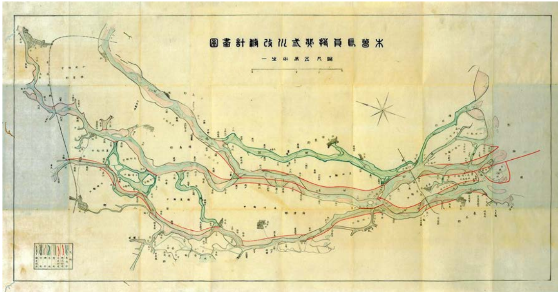
Figure 4: Kiso Nagara Ibi. Three Rivers Improvement Plan (1900). North is to the left side; the rivers flow from left to right on this map. Gifu City is shown in the upper left corner. This map was drawn in 1/50,000 scale, based on the large map of Johannis De Rijke in 1/10,000. [housed in the Gifu Prefectural Historical Museum]
