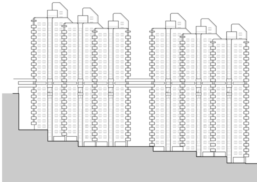
Figure 2. Transforming the High-rise into the Multistory with the Corridor by Taking Advantage of Mountainous Topography
