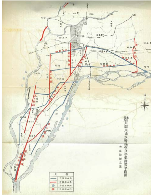
Figure 5: Akira Kira. Irrigation/Drainage Trunk Channel Improvement Plan for the Area between the Kiso and Nagara Rivers (1924). Blue and red lines indicate irrigation and drainage channels respectively. The streams are of Nagara River (upper) and of Kiso River (lower). The upper hatched area is downtown Gifu City. [Ohno, 1933]
