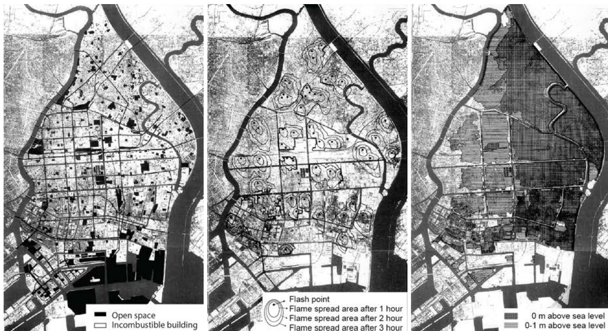
Figure 1: Open space and incombustible building, Flame spreading model and Flood area in Koto-delta researched by Takayama laboratory.
