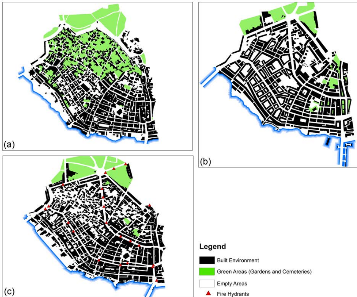
Figure 7: Schemes of Galata in terms of built environment and green areas according to old maps using the methods integrated to Geographic Information Systems (ArcGIS 4.1 Software): (a) Ostoya Map, (b) Huber Map, (c) Goad Map
