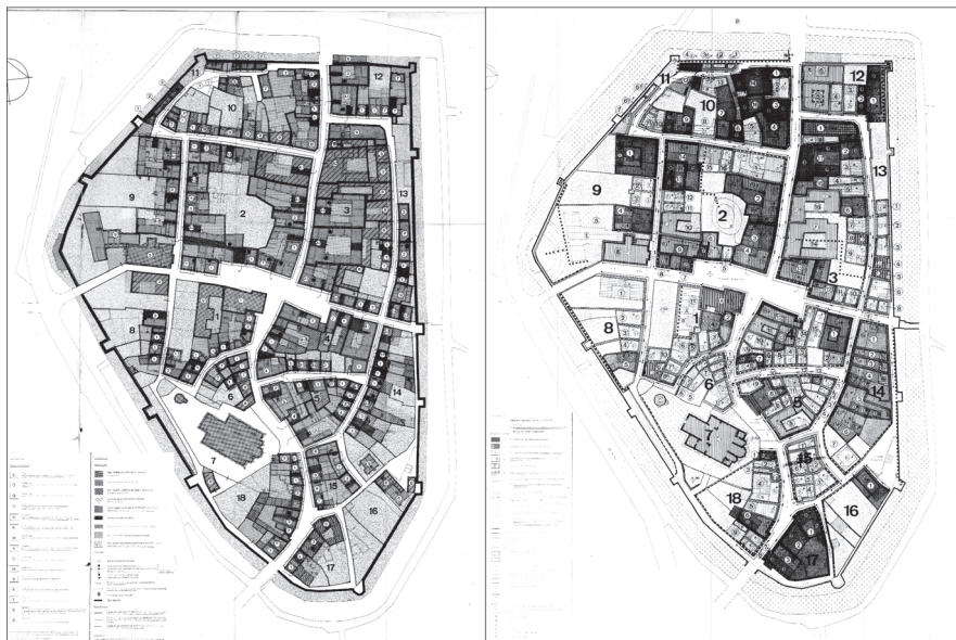
Fig. 3. Typological classification (left) and operational reconstruction plan with the intervention categories (right). Source: Venzone Municipal archives.
