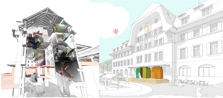
Fig. 4. A - Representations of the digital twin. Left, section through: topographic model, point cloud -geomaticians-, SBB infrastructure model -engineers-, architect model existing (black) and transformed (red) e.g. allowing access to people with reduced mobility. B - Architect's view of the transformation. Beyond the graphic aspect, the building's geometry is represented with 1cm tolerance and the shadow projection is exact (21.09.17/12:00).
