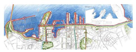
Figure 3 Masterplan showing pedestrian promenade, cycle and light rail routes, and proposed linking bridges
