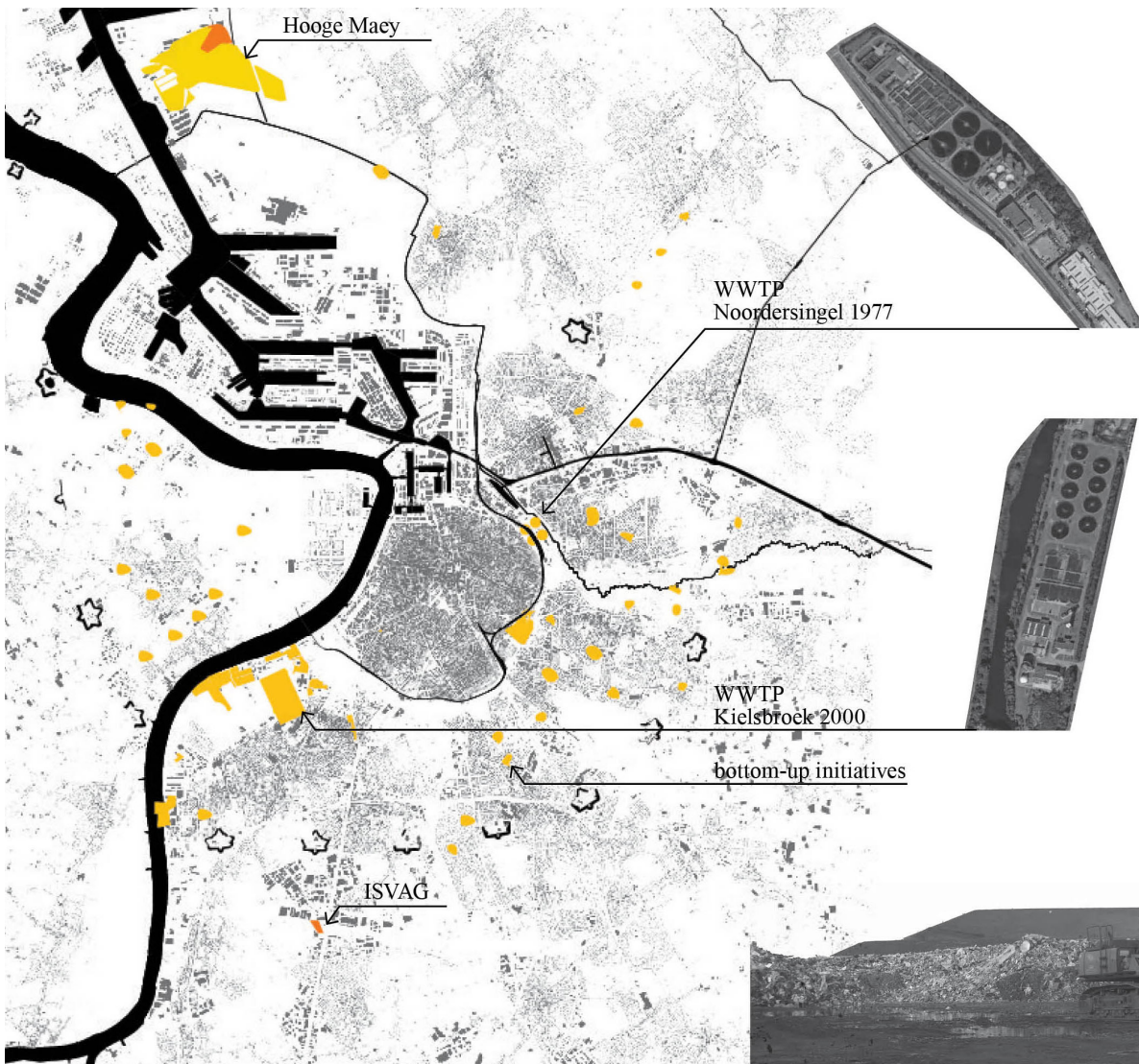
FIGURE 6 (situation 2015) As a result of waste centralisation policies, Antwerp's waste processing facilities are composed of a series of outer city waste hubs that combine different waste related infrastructures such as waste water treatment plants and municipal recycling parks. Picture: Hooge Maey.
