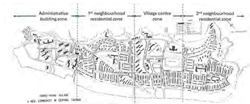
Fig. 2. The Layout of Main Buildings and Zoning Division of JNV Urban Plan. Source: revised the chart from EHEO, The Comprehensive Report, 153.
