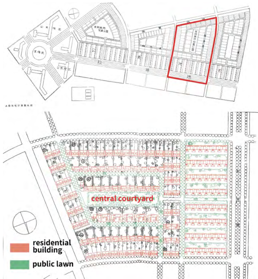
Fig. 2. master plan of the Oriental Development Company residential district. The central courtyard becomes the public space of the low-rise residential district. The green promenade between the multi-unit dwellings is open to the outside, connecting the main road and the residential district.
