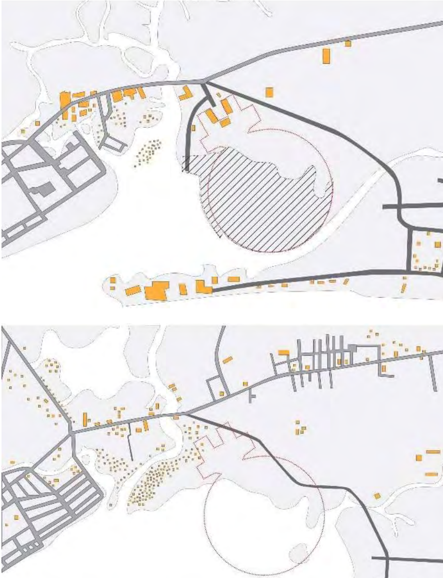
Fig. 1. Comparison between 1914 map (Above) and 1930 map (Below) for the extent of land reclamation (339 acres) in the construction of the civil aerodrome (DPA).
