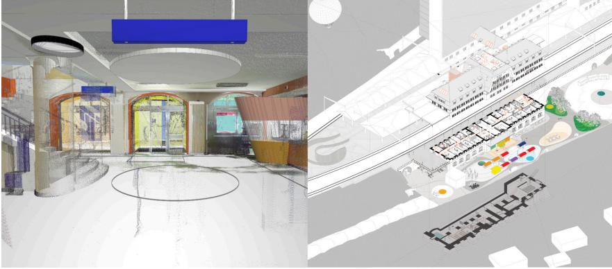
Fig. 6. A – Federation of point cloud and architectural model after transformation: view in the majestic hall toward entrance with fictive information desk. Point clouds demonstrate the accuracy of the architectural model. B – Exploded isometric of the design: the precision of the point cloud allows exact modelling and highly precise transformations simulations to the benefit of conservation.
