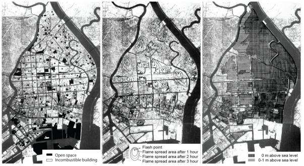
Figure 1:Open apace and incomustible building, Flame spreading model and Flood area in Koto-delta researched by Takayama laboratory.
