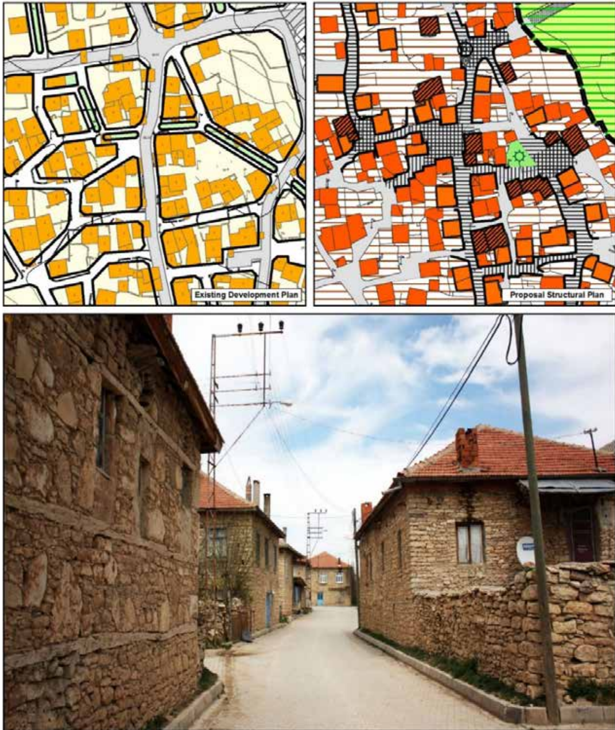
FIGURE 3 Pedestrian paths should be at least 10 meters in width and carriageways should be at least 12 meters according to legal regulations in Turkey. This arrangement/rule concerning road widths is one of the most important reasons behind the corruption of settlement patterns in rural areas.
