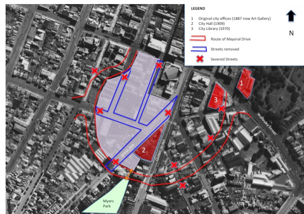
FIGURE 4 The city engineer's plan for Quadrant Road (later renamed Mayoral Drive) and its extension to the south and east of the civic centre.
