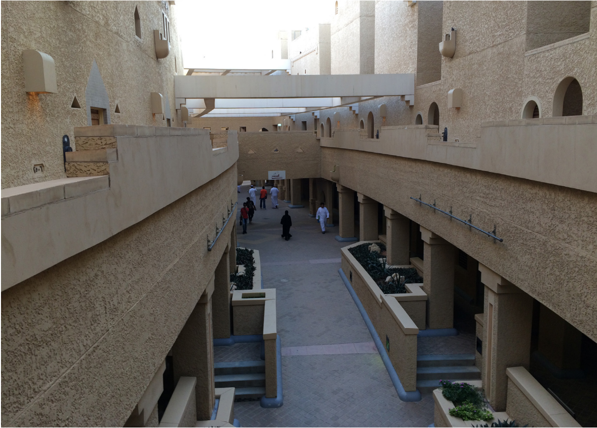
FIGURE 7 Major Core's pedestrian connection. Townhouses are accessible only from the first level. Even at that level, privacy and climate control is kept as much as possible, avoiding large openings.
