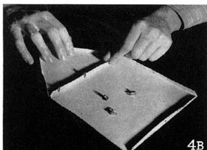
4B PINCH CLIPS , easy to apply, permit disassembly of globe. If clips are used last segment must be taped or glued in.
