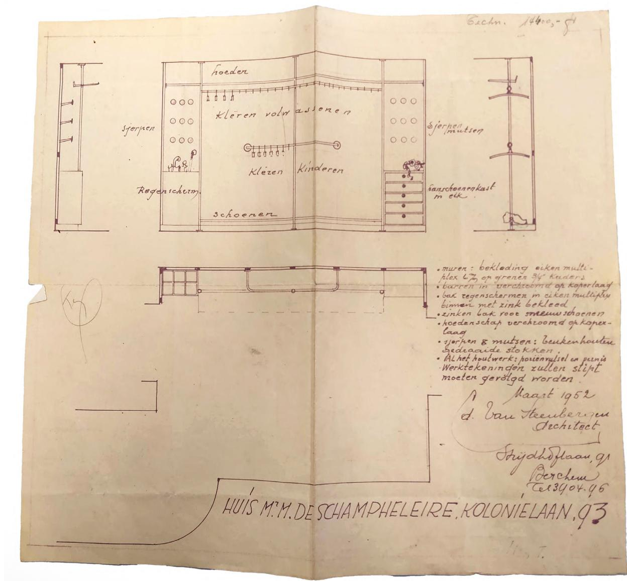
Fig. 7: Eduard van Steenbergen, design of a wardrobe with instructions. Source: VAI.
