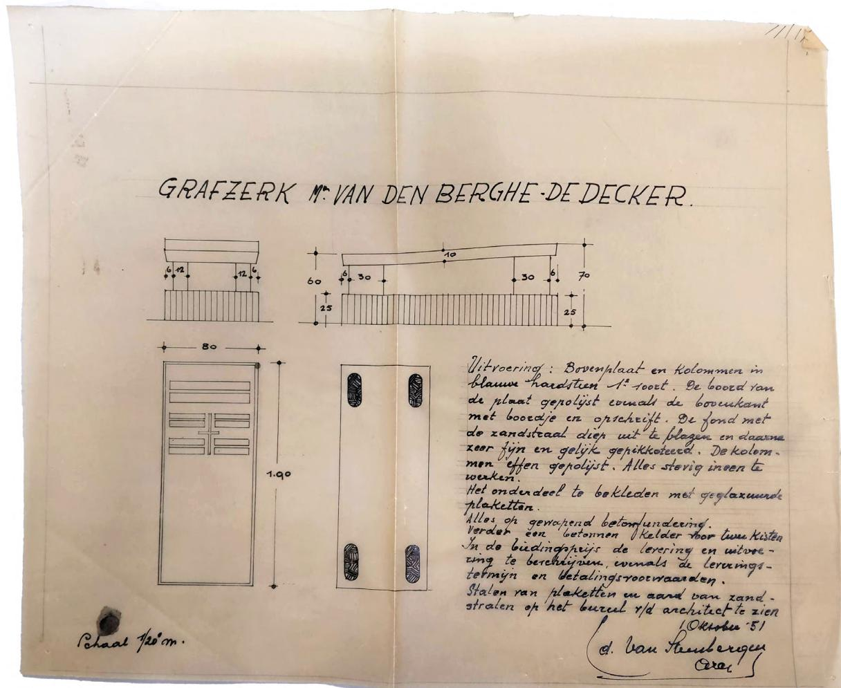
Fig. 6: Eduard van Steenbergen, gravestone design with instructions. Source: VAI.
