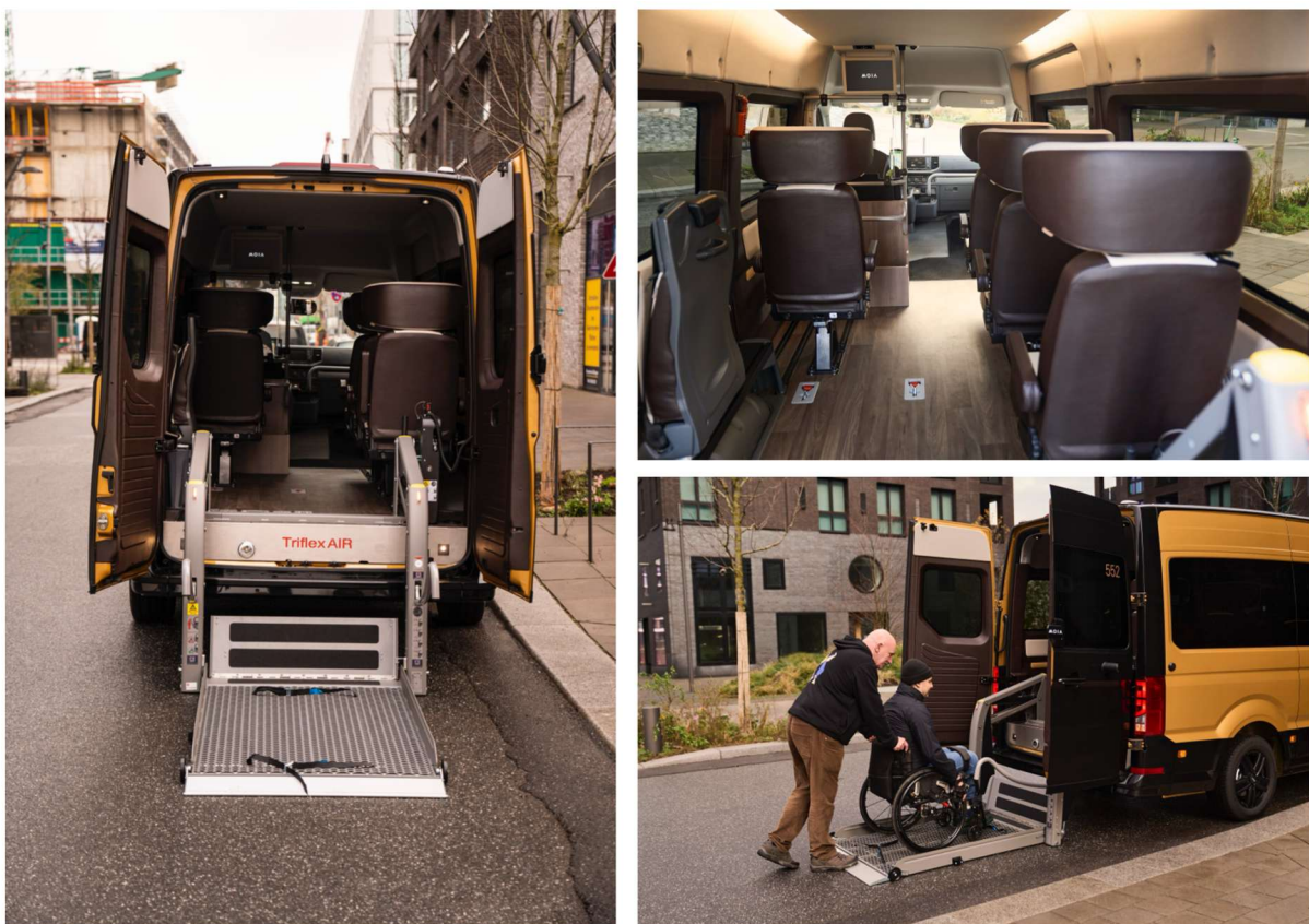
Figure 1. Impressions of MOIA's wheelchair-accessible vehicle with rear lift and four additional seats.
