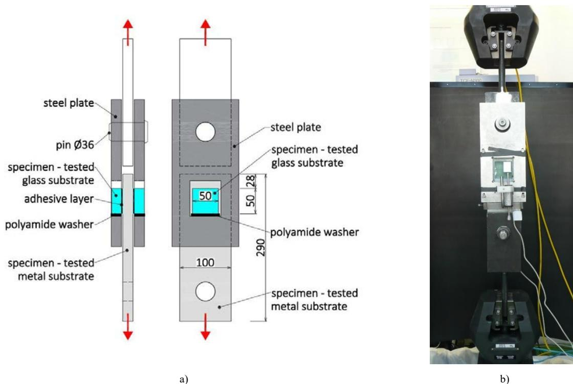
Fig. 2a) Schema of double lap shear joint, b) Specimen in machine.
