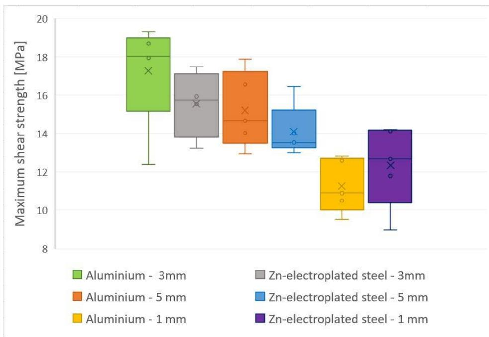
Fig. 5 Maximum shear strength for reference set of specimens.
