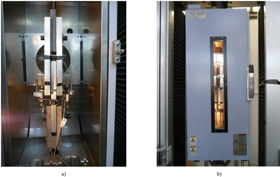
Fig. 4a) Specimen in the temperature chamber b) Temperature chamber.
