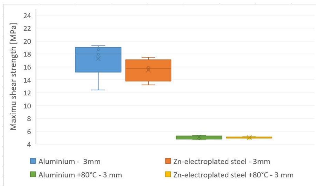
Fig. 8 Maximum shear strength for specimen at room and elevated temperature.
