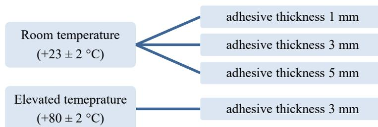
Fig. 1 Sets of specimens.
