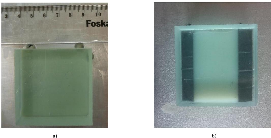
Fig. 3a) Specimen with glass balls, b) Specimen with foam tape.
