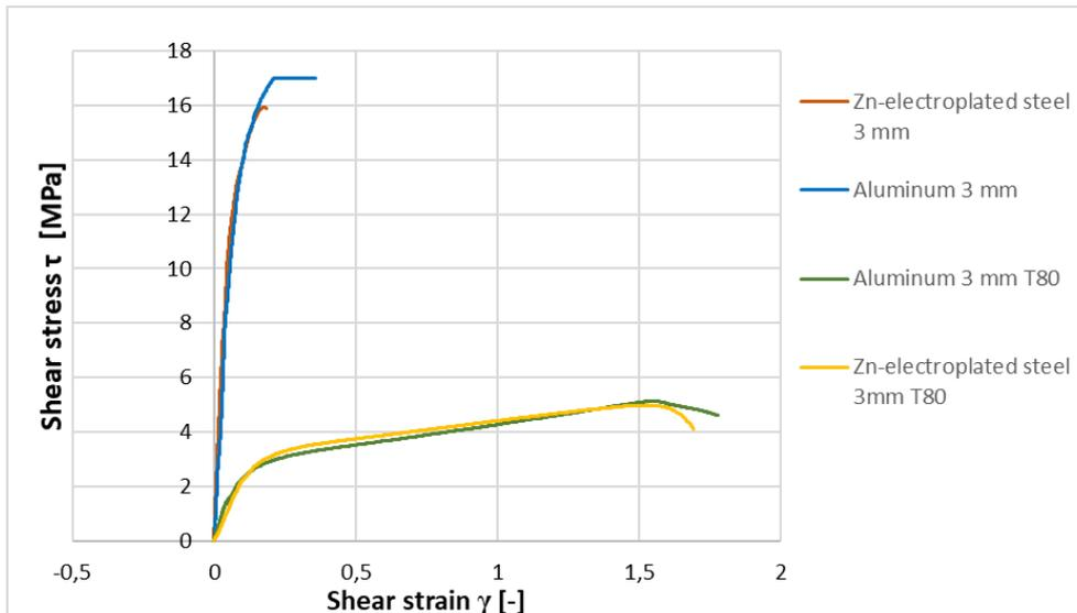
Fig. 7 Stress-strain relationship for specimens at room and elevated temperature.
