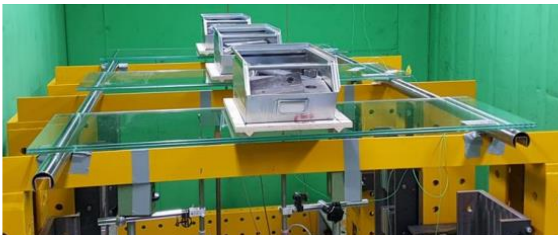
Fig. 2 Four-point bending verification set-up in temperature chamber (picture courtesy of Institute of Structural Engineering, University of the German Armed Forces, München, Germany).
