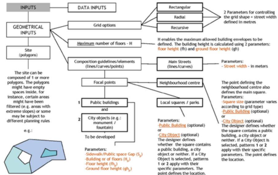
Figure 41 Geometrical inputs.
