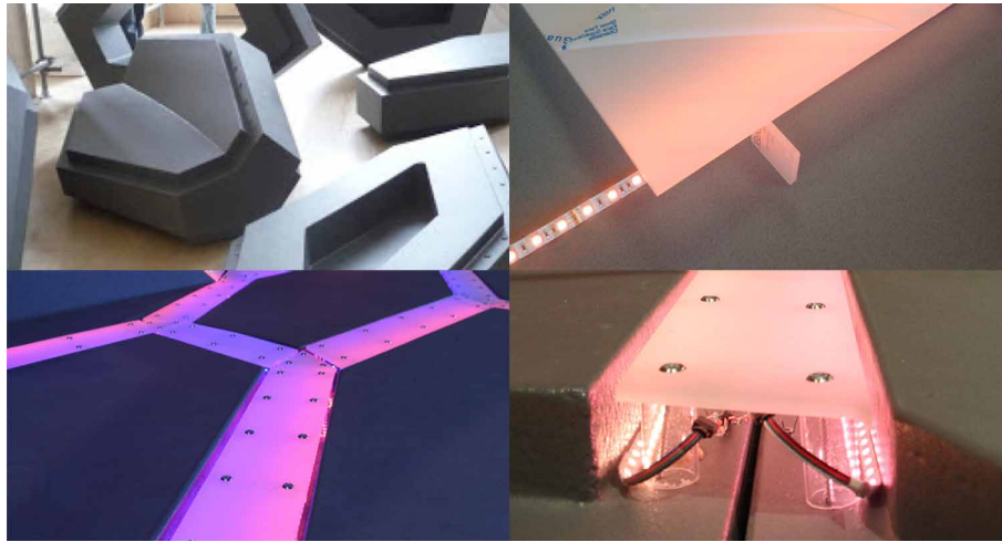
FIG. 4.3 Top: Single protoCELLs (Left); testing Perspex® over LED1 (Right). Bottom: Generated color gradient (Left); Acrylic connections & two LED-strips within the seam of two protoCELLs (Right).
