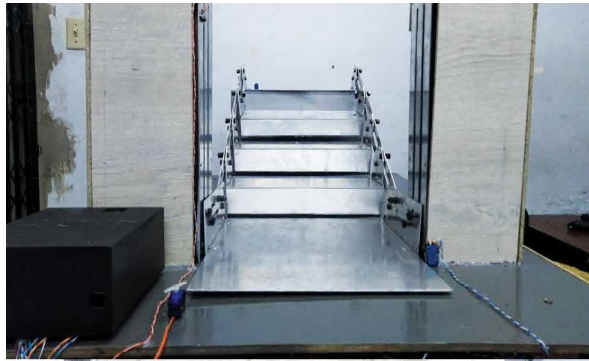
FIG. 5.42 Variation 2 configured for ( Top and Middle ) the 1st user-type (standard-stairs); and ( Bottom ) the 3rd user-type (elevating platform).
