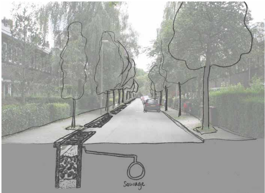
FIGURE 8.11 Existing street (1) and impression of water infiltration units (2).
