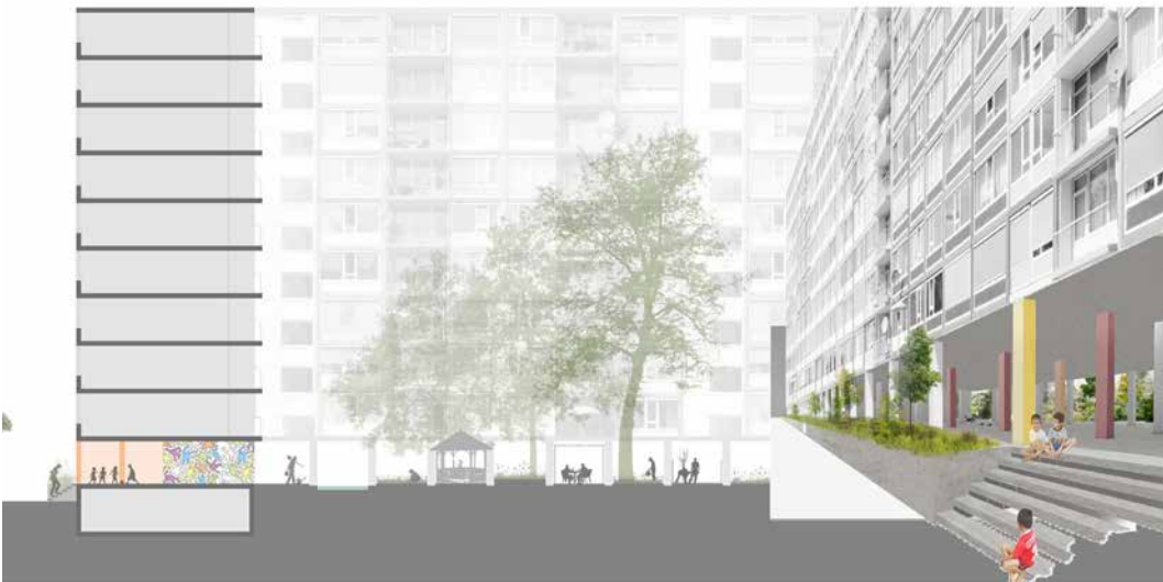
FIGURE 8.51 Opening up the ground floor for ventilation and sheltered community space by Frederico Lia (Schrijver et al., 2014)
