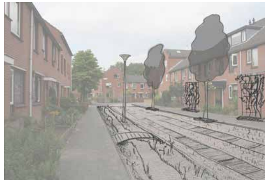
FIGURE 8.35 1. Existing street with parking; 2. Impression of a street with calm traffic due to a narrow trail next to grass tiles, wadi and street trees.
