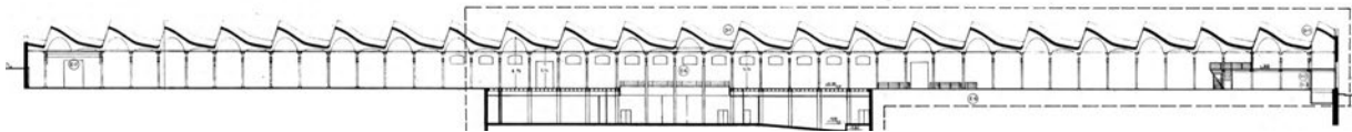
FIG. 11.3 Section of the former production hall with the underground extension and the administration mezzanine (mNACTEC documentation centre).
